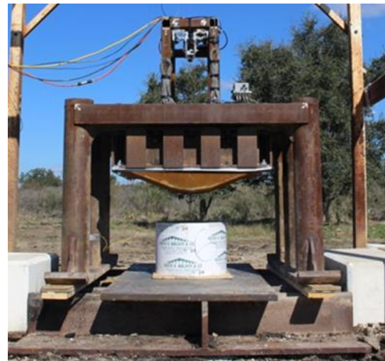
Figure 4: SwRI's Landmine Test Fixture holding a bilinear V hull component above a soil pot. At the top of the test fixture is the superstructure holding dual offset high-resolution high-speed cameras.
